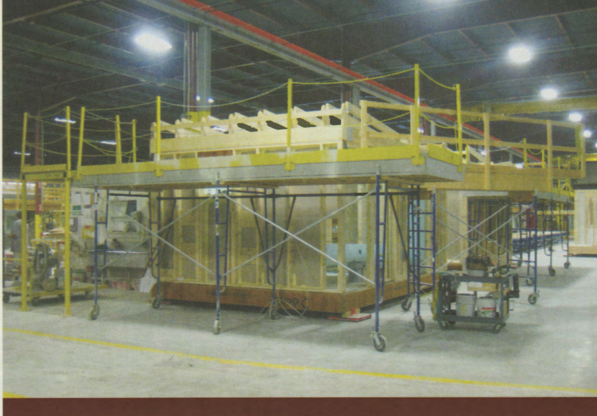
The modular-home components were built in the Preferred Building Systems factory.
